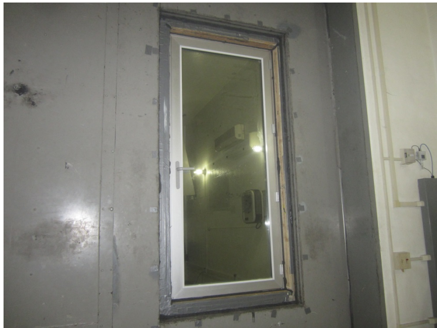
Source Room View of Installed Specimen
